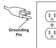
125 V~ 3-Prong Plug and Outlet (for up to 125 V~ and up to 15 A)
